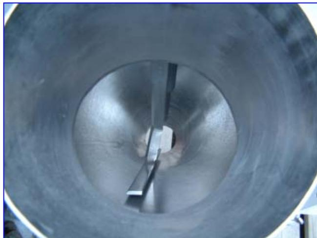
Use the following to locate and identify parts and tooling configurations used with auger filling machines. Free flow tooling is used with free flowing powders such as granulated sugar, salt, bread crumbs, etc. Non free flowing tooling is used for products such as bakery mixes, carbon, talcum powders, etc.
