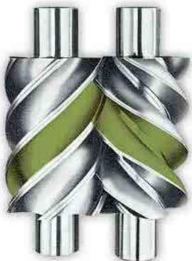
**Compression Phase** — As rotation continues, the gas in the interlobe space is carried around the circumference of the compressor housing. Further rotation meshes male and female lobes thus reducing interlobe volume. Positive displacement compression continues in the direction of the discharge port.
