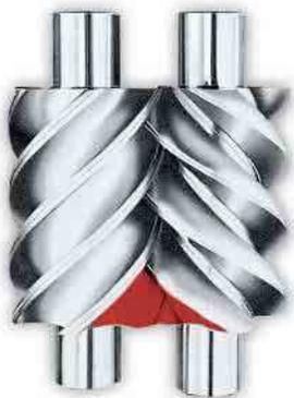
**Discharge Phase** — At a point determined by the designed “built-in” compressor volume ratio ( $V$ ), the discharge port is uncovered and the compressed gas is discharged by further meshing of the male and female interlobe space. While the meshing point of a pair of lobes is moving axially, the next charge is being drawn into the unmeshed portion and the working phase of the compressor cycle are repeated.
