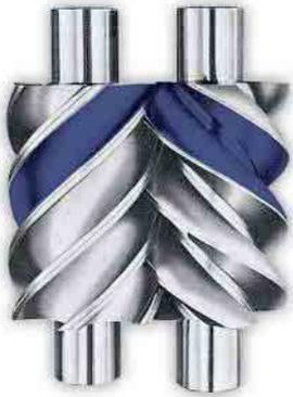
**Suction Phase** — As a lobe of the male rotor begins to unmesh from an interlobe space in the female rotor, a void is created and suction gas is drawn in through the inlet port. As the rotors continue to turn the interlobe space increases in size, and gas flows continuously into the compressor. Suction is sealed off when the interlobe space reaches its maximum volume.
