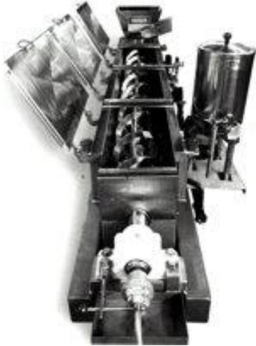
Groen Continuous Screw Blender and Coater. Model CSB. Is idea for coating popcorn and can be used to process a variety of products requiring continuous mixing and uniform coating. The Model CSB can be sized to meet your product residence time and throughput requirements and is equipped with an appropriate flight screw for proper particulate mixing and coating action. The trough shaped shell is normally fitted with a high pressure jacket, designed for either heating or cooling applications.
