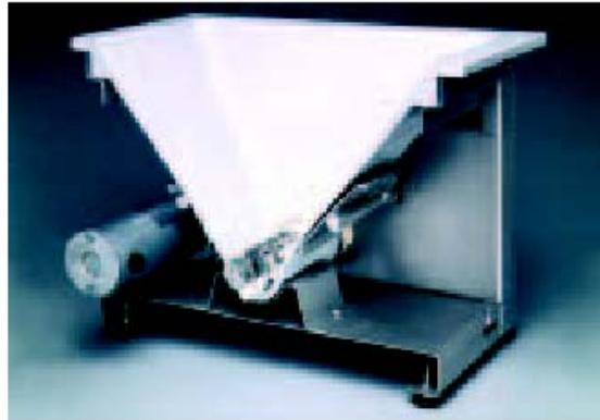
Volumetric metering deviations generally range from  $\pm .5$  to 3% for most materials. Loss-in-weight feeding systems are available for even more precise accuracies. (See back for testing information.)
