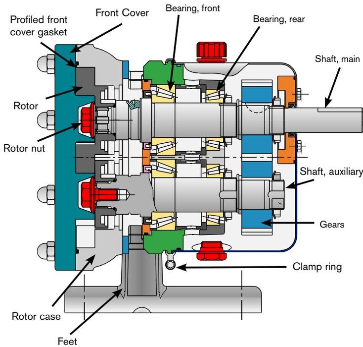
Expanding cavities are formed at the inlet drawing the liquid into the rotors. Meshing of the rotors forces the fluid out of the pumping chamber.
