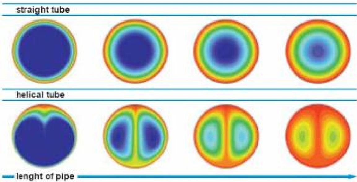
The figures above show the heat distribution of a fluid flowing in a straight tube and a curved tube in relation to tube length. The wall temperature is 100°C, the tube diameter is 0.025 meters and the rate of flow is 1 meter/sec. The situation is shown after 1 meter, 30 meters, 100 meters and 200 meters. Blue, green, yellow and red indicate the rising temperature.
