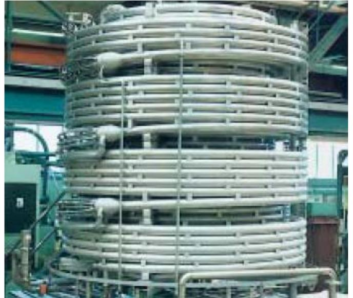
Multi-tube heat exchangers used in high capacity UHT plants
