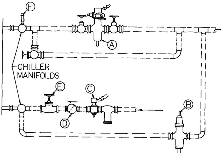
**Control Includes:** Combination suction pressure regulator stop valve with pressure gauge; relief (defrost) valve; liquid solenoid valve with strainer; check valve; hand expansion valve; manifold relief valve; full suction by-pass.
