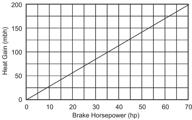
$$\text{Fan Temperature rise} = \frac{(\text{Fan Heat (Mbh)})}{(1.085 \times \text{Fan cfm})}$$
