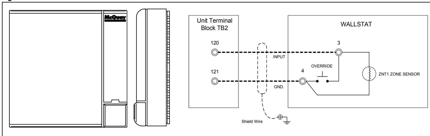
Figure 8: Zone sensor with tenant override and remote set point adjustment
