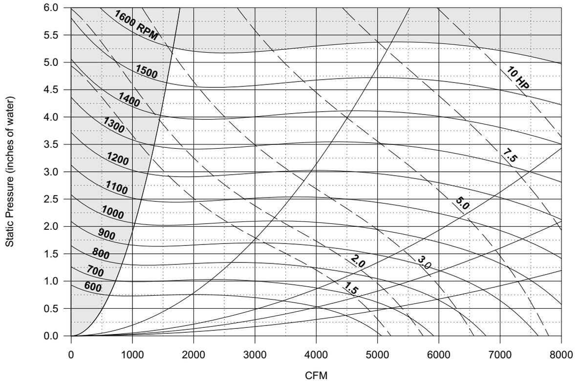
Figure 25. SWT023C/028C, 18"x18" Fan, without Variable Inlet Vanes
