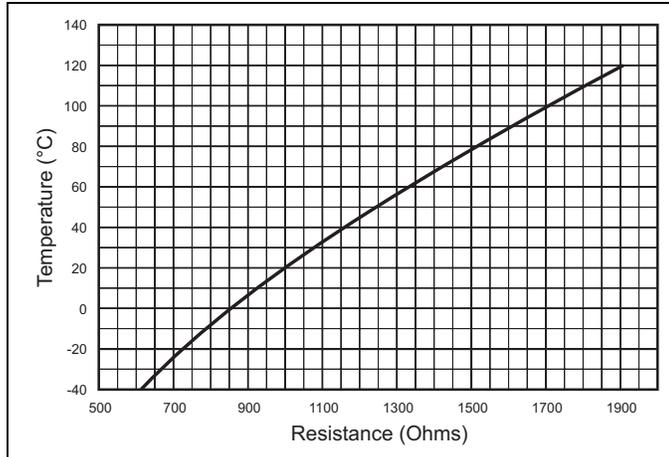
**Table 25: MicroTech II temperature sensor—temperature vs. resistance chart**
