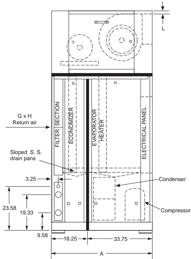
Figure 29. Left Side, Back (CCW) Discharge
