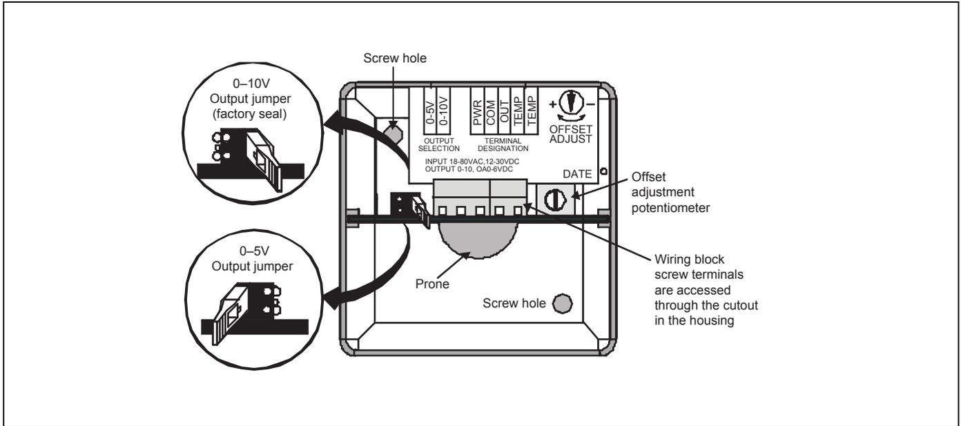
**Figure 11: Humidity sensors (wall mounted)**
