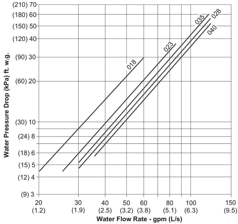
Note: Includes coil, control valve and interconnecting piping.
