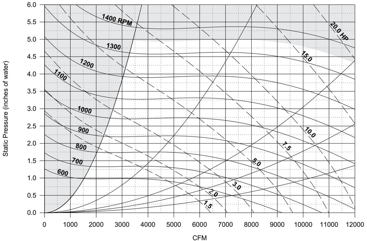
Figure 27. SWT 035C/040C. Dual 15"x15" Fan, Without Variable Inlet Vanes
