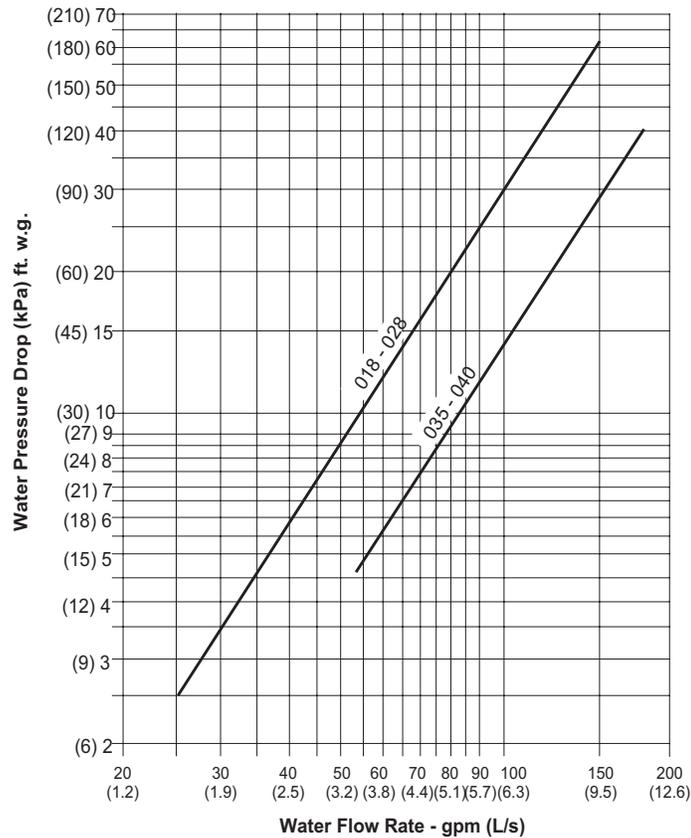
Note: Includes coil, Control valves, and interconnecting piping.
