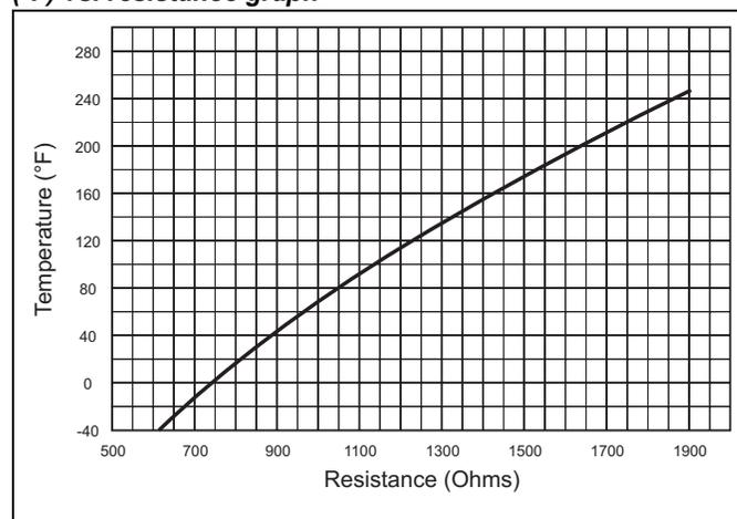
**Figure 25: MicroTech II temperature sensor—temperature (°C) vs. resistance graph**
