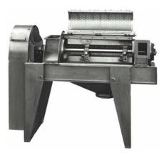
**VERSATILITY:** By changing screens (hole size), paddle speed, pitch, clearance, rpm, and feed rate, it is possible to pulp, finish, or de-water a wide variety of fruits, vegetables, and other products, and to obtain maximum yield consistent with finished product specifications.
