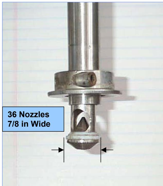
US Bottlers VF-36 Head Pressure Filler, gal set-up, star infeed-discharge, 0.875in D nozzle, 5.75in centers, configurable heads, 0.75hp vari-speed drive, 75in W x 92in H x 95in L.
