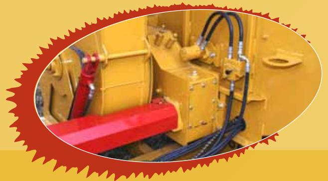
**Fan:** The new fan design is welded on a HD 2 inch shaft for improved fan output. The fan housing and discharge chute is lined with AR 400 high abrasion steel for long life and improved performance. Both horizontal and vertical articulation is accomplished by hydraulics controlled from the tractor cab with a joystick control.
