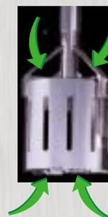
The two high-velocity, counter-current streams converge within the stator causing high turbulence and hydraulic shear, without momentum loss from obstructions within the stator.
