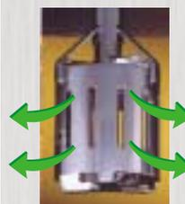
The high velocity radial discharge combines with slower moving tank flow for additional hydraulic shear and circulation.
