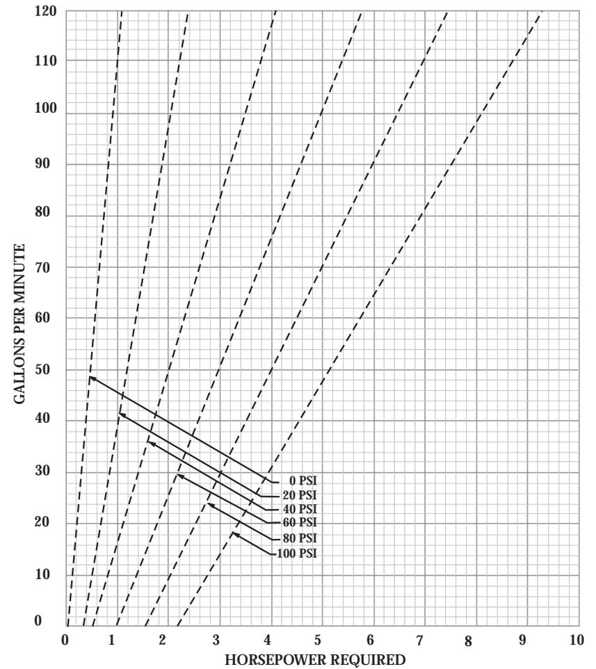
Note: This graph is predicated upon liquids of the viscosity and specific gravity of water and milk at 100°F (34°C). The horsepower ratings are actual brake horsepower. This graph applies to polymer coated rotors only.
