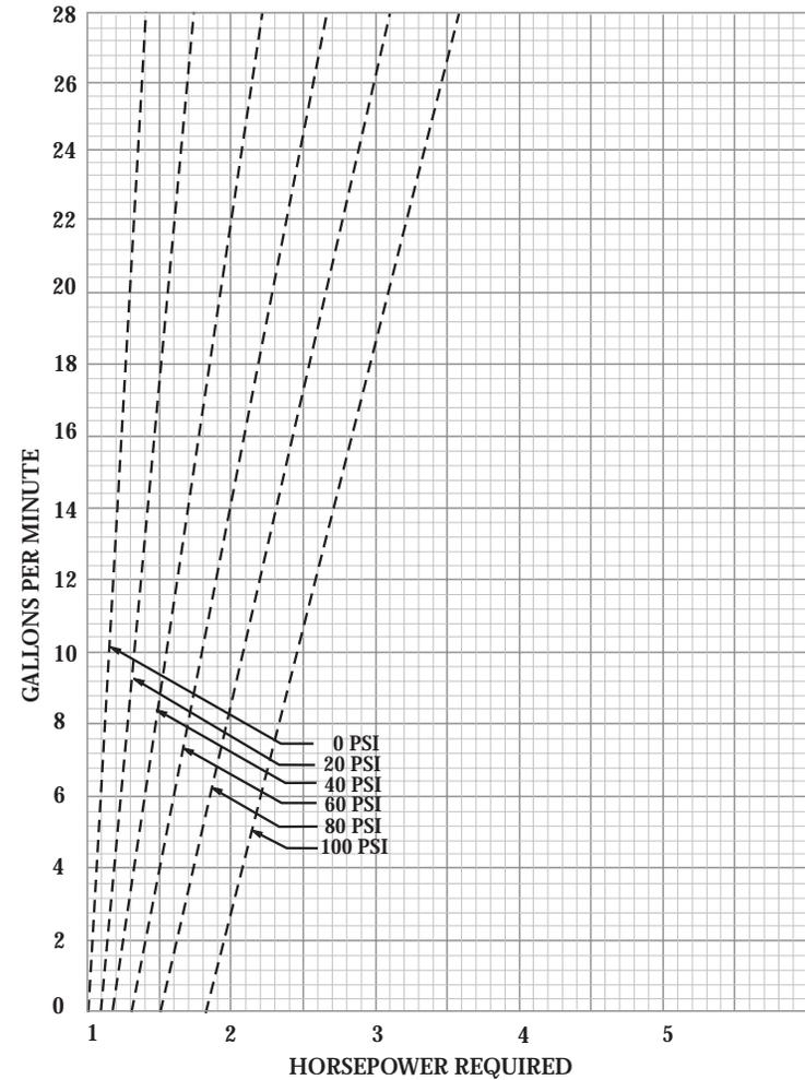
Note: This graph is predicated upon liquids of the viscosity and specific gravity of water and milk at 100°F (34°C). The horsepower ratings are actual brake horsepower. This graph applies to polymer coated rotors only.
