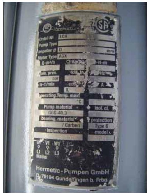
Hansen Technologies Hermetic Centrifugal Pump. Model: 1997. S/N: CH-82786. Order No: LCH82786. Type: CAM2/3. Maximum capacity: 52.7 gpm @ 138 tdh. Minimum capacity: 4.39 gpm @ 203 tdh. Impeller diameter: 4.48/5.11 in. Nominal pressure: 362 psi. Power supply: 4 hp (3.0 kW), 3400 rpm, 440 V, 7.5 amps, 60 Hz, 3 phase. Inlets: (1) 1-1/2 in. dia. flanged port. Outlets: (1) 1 in. dia. flanged port. Overall dimensions: 2 ft. L x 9 in. W x 10 in. H.
