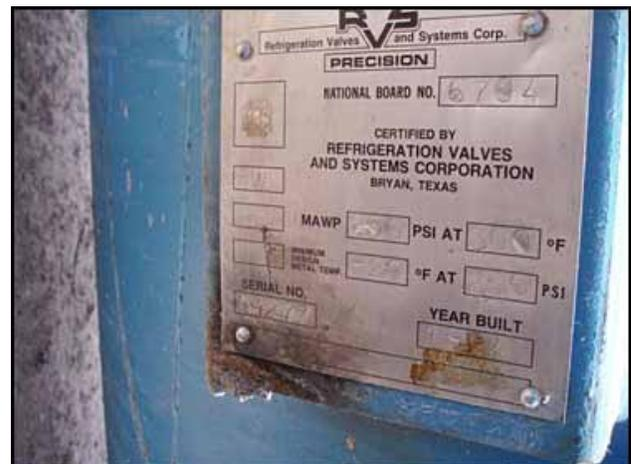
1994 Refrigeration Valves & Systems Vertical Receiver- 18 Gallon. S/N: 94407. Nat'l Bd: 6754. Inside straight-wall dimensions: 1 ft. 1 in. dia. x 2 ft. 8 in. H. MAWP: 250 psi @ 300°F. MDMT: -20°F @ 250 psi. Inlets: (1) 1/2 in. dia. port, (1) 1 in. dia. port. Outlets: (1) 1/2 in. dia. port, (1) 1 in. dia. drain port, (2) 1 in. dia. ports (relief) (1) 1-1/2 in. dia. port. Overall dimensions: 3 ft. 7 in. L x 3 ft. 4 in. W x 6 ft. 4 in. H.
