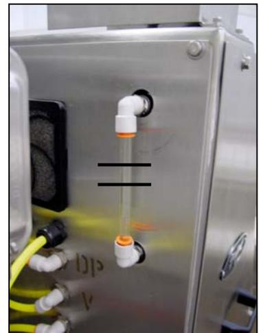
**CAUTION:** Low water level inside the water jacket may result in heater failure.
