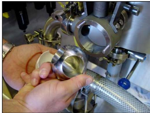
3. Inspect the housing and valve ball actuator tab before reassembly.
