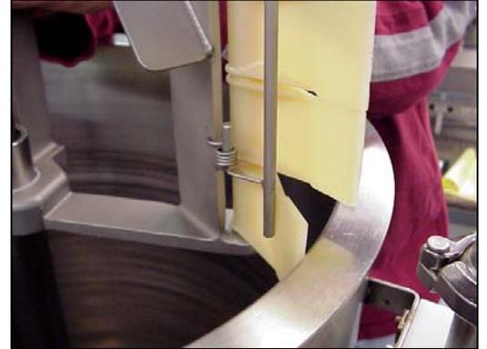
6. Clean any remaining product from tank, agitator assembly and melting rack. Rinse with clean water.
