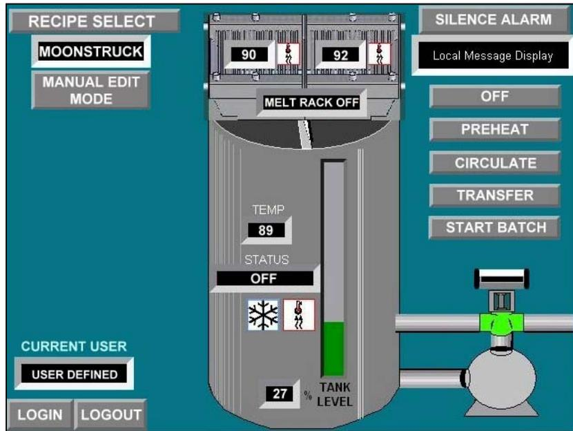
Use the function keys to select the desired machine function. Once the desired function is selected a 5 second wait period is required for the function to initiate.
