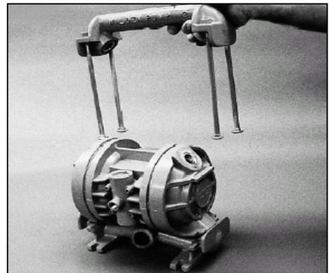
3. Remove the discharge valve balls, seats and O-rings from the top manifold and inspect for damage or wear. Note: Teflon O-rings should be replaced when reassembled.
