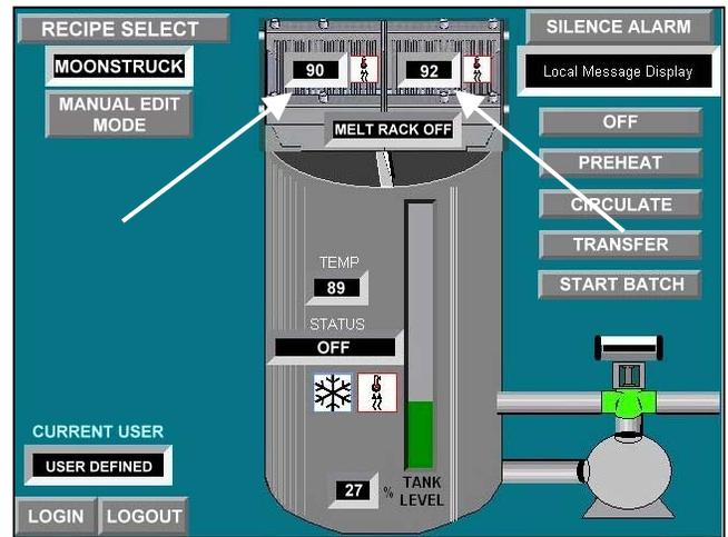
2. Touch the "SET TEMP" box to modify the temperature setting. This box is ONLY accessible when in the "MANUAL MODE".
