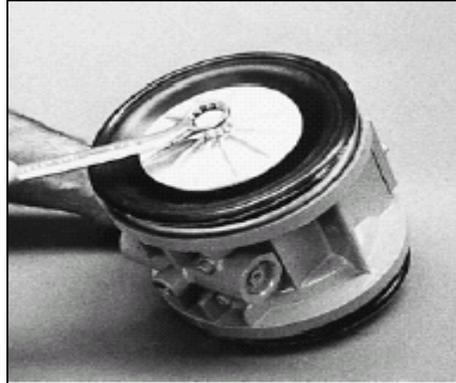
6. Note: One of the following two situations may occur. (1) The outer piston, diaphragm and inner piston remain attached to the shaft and the entire assembly can be removed from the center section. (2) The outer piston, diaphragm, inner piston and disc spring separate from the shaft which remains connected to the opposite side diaphragm assembly. NOTE: Teflon-fitted pumps come standard with back-up diaphragms (not shown).
