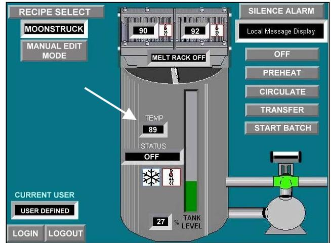
2. Touch the “SET TEMP” box to modify temperature setting. To turn the tank chiller and tank heater “OFF” or “ON”, touch the respective “ICON” (see arrows) and follow pop-up screen instructions.
