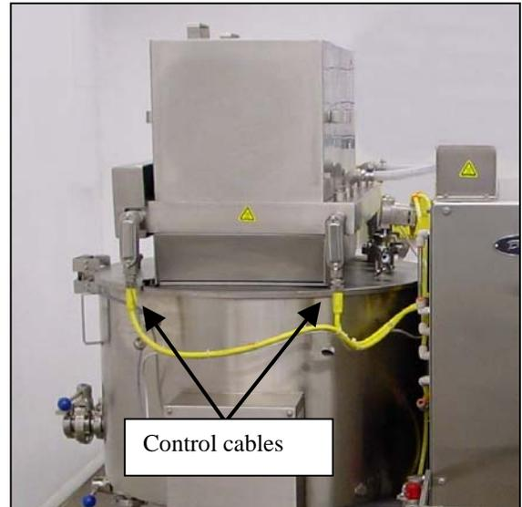
2. With assistance, lift the melting rack from product tank.
