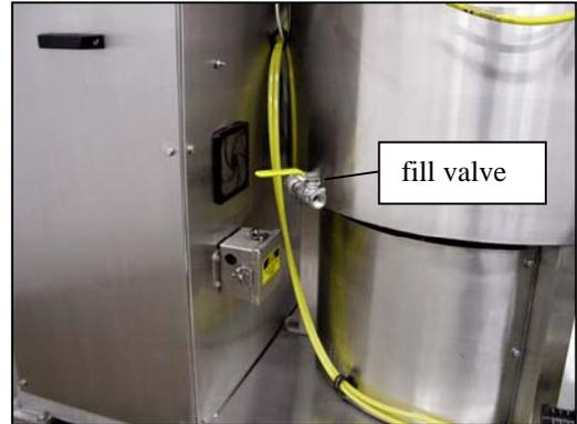
4. Close yellow water valve when water level reaches the sight tube. Touch “CIRCULATE” from the operator panel. This will operate the circulating pump. Add or remove water until sight tube is half full while the circulating pump is running. **IMPORTANT:** If the water jacket is completely filled the water jacket will not vent properly during machine operation.
