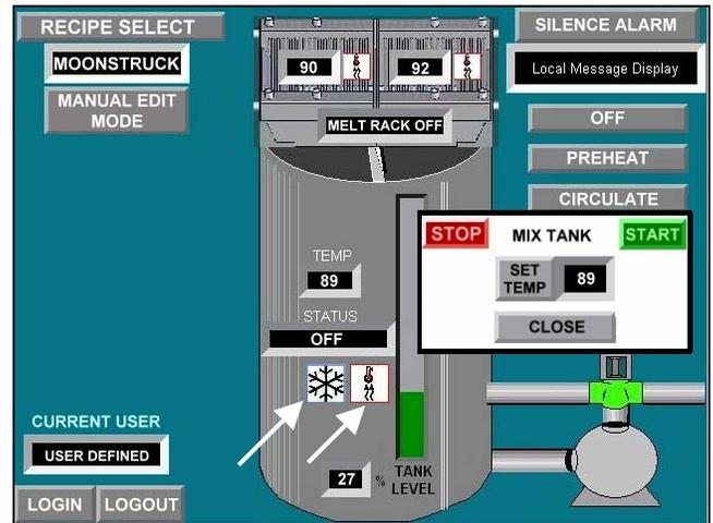
**NOTE:** This value is the temperature of the circulating water in the tank water jacket, NOT the actual product temperature.
