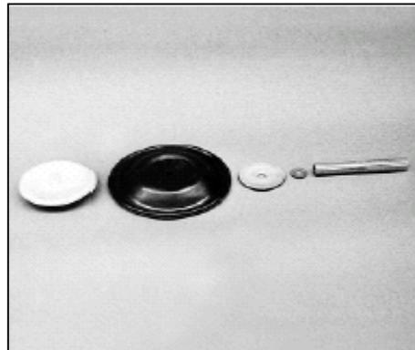
7. To remove the diaphragm assembly from the shaft, secure the shaft with soft jaws (a vise fitted with plywood or other suitable material) to ensure the shaft is not damaged. Using an adjustable wrench, remove the diaphragm assembly from the shaft.
