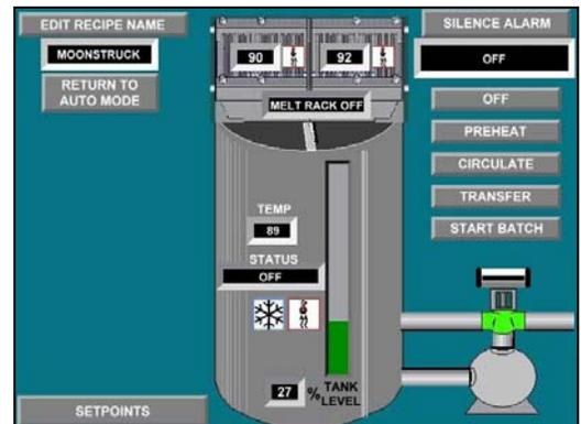
**NOTE:** All changes made to the machine “SETPOINTS” will be saved to the recipe name shown in the upper left corner of the screen.
