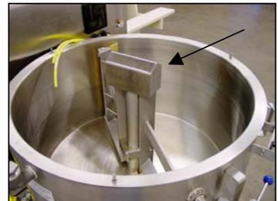
4. Loosen agitator setscrews on both sides of the agitator shaft.
