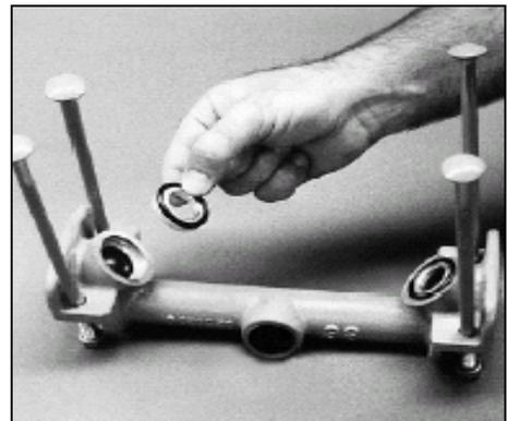
4. Remove the valve seat, valve seat O-ring and valve ball from the bottom manifold and inspect for damage or wear. Note: Teflon O-rings should be replaced when reassembled.
