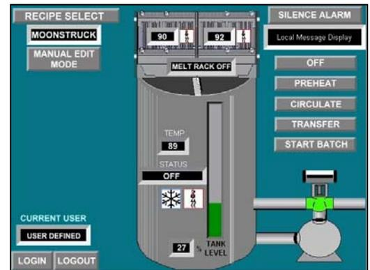
4. Once butter has been melted and of desired consistency, select the “TRANSFER” function. This function will maintain the mix as the Arcall Slinger signals for more product.
