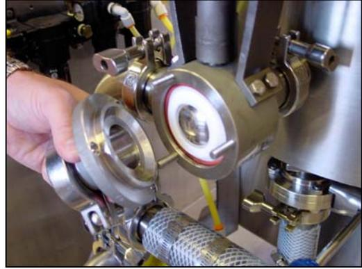
2. Remove O-Ring, valve ball bushing and valve ball; then inspect for damage or wear. NOTE: Use care when removing these items.
