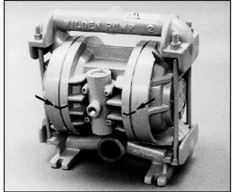
2. Remove the four long carriage bolts that secure the top and bottom manifolds to the center section. Remove the top manifold and lift the center section off the bottom manifold.
