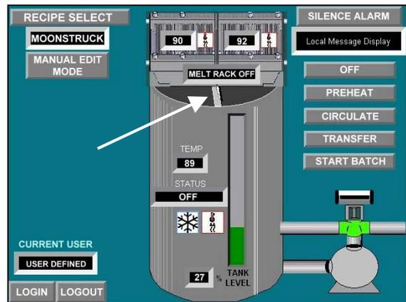
The agitator is only operational when activated via “ICON” located on the panelview display.
