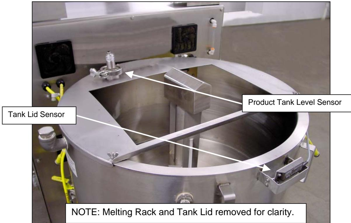
**WARNING:** Do not depress the small white button on the product tank level sensor. Sensor failure may result.
