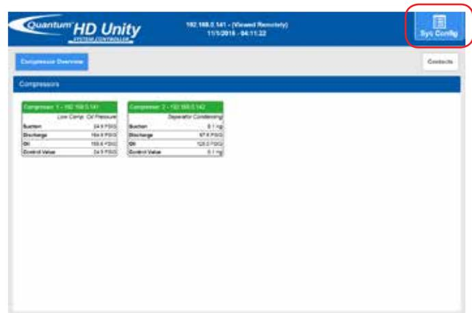
Selecting this button will cause the system configuration menu (which is determined by your assigned access level) to be superimposed over the current screen.
