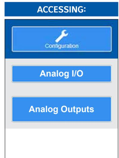
**DESCRIPTION:** The Analog Outputs screen is used to view and set the Analog Output I/O board and I/O channel assignments:
