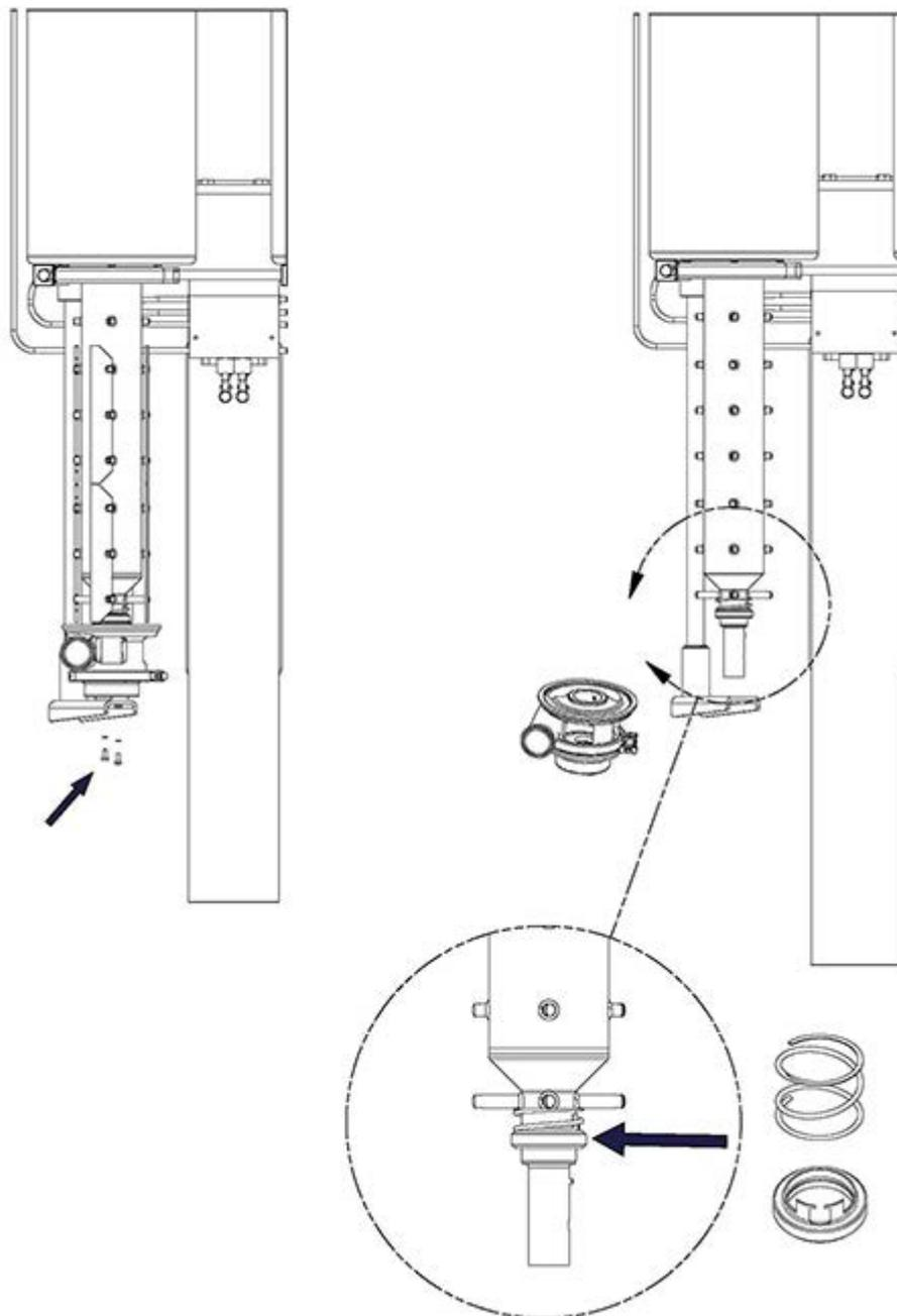
Figure 7-2B. Using Helper Plate to Access Lower Head & Seal Components
