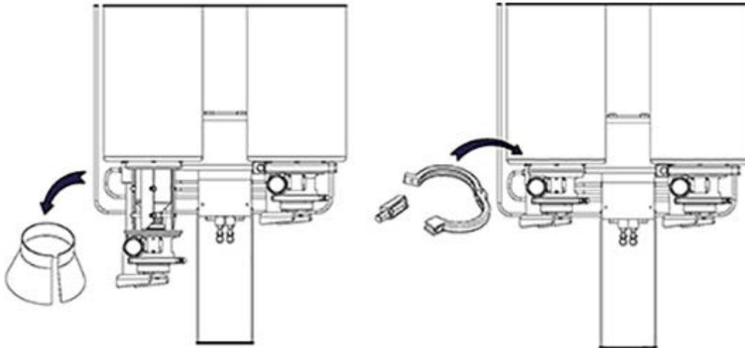
Figure 8-8C. Removing the Blade Funnel
