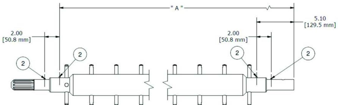
**Figure 8-4. Seal Pin Locations for Rotors with External Lower Bearings**
