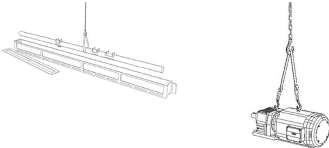
Figure 6-3. Take caution to properly and safely lift Contherm™ from Crate
