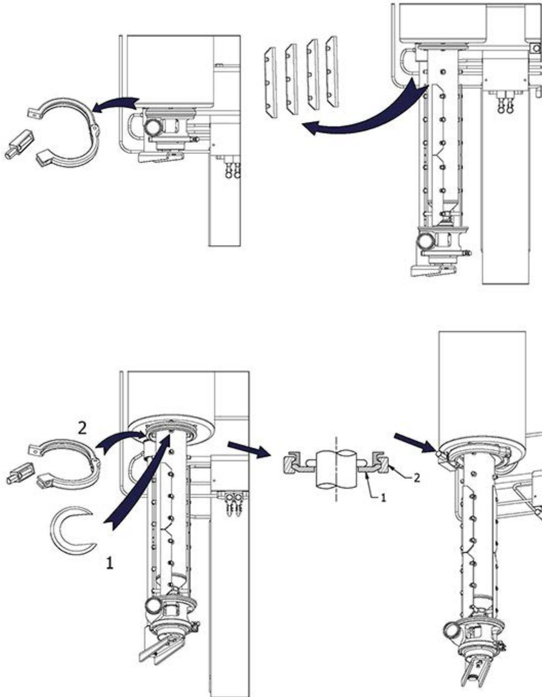
Figure 7-2A. Installing the Rotor Helper Plate
