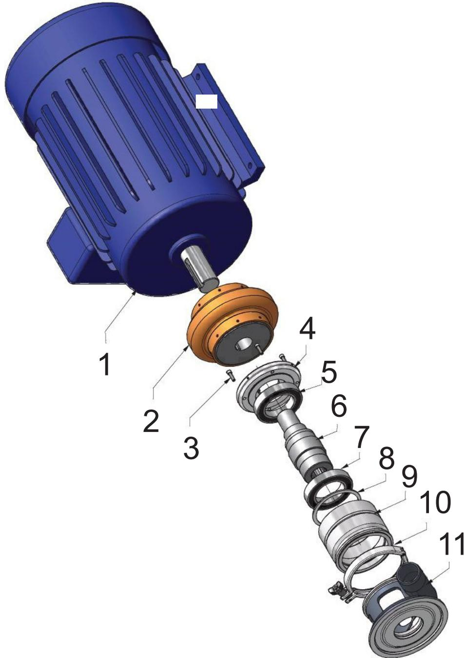
Figure 8-13. Upper Bearings, Direct Coupled, Electric Drive Motor
