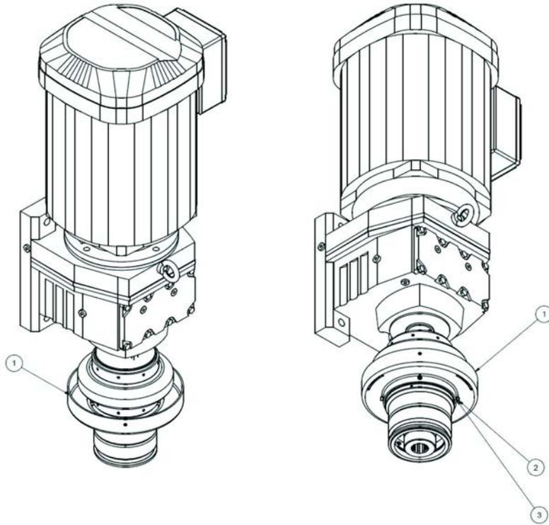
Figure 6-11A Installing the coupling guard.
