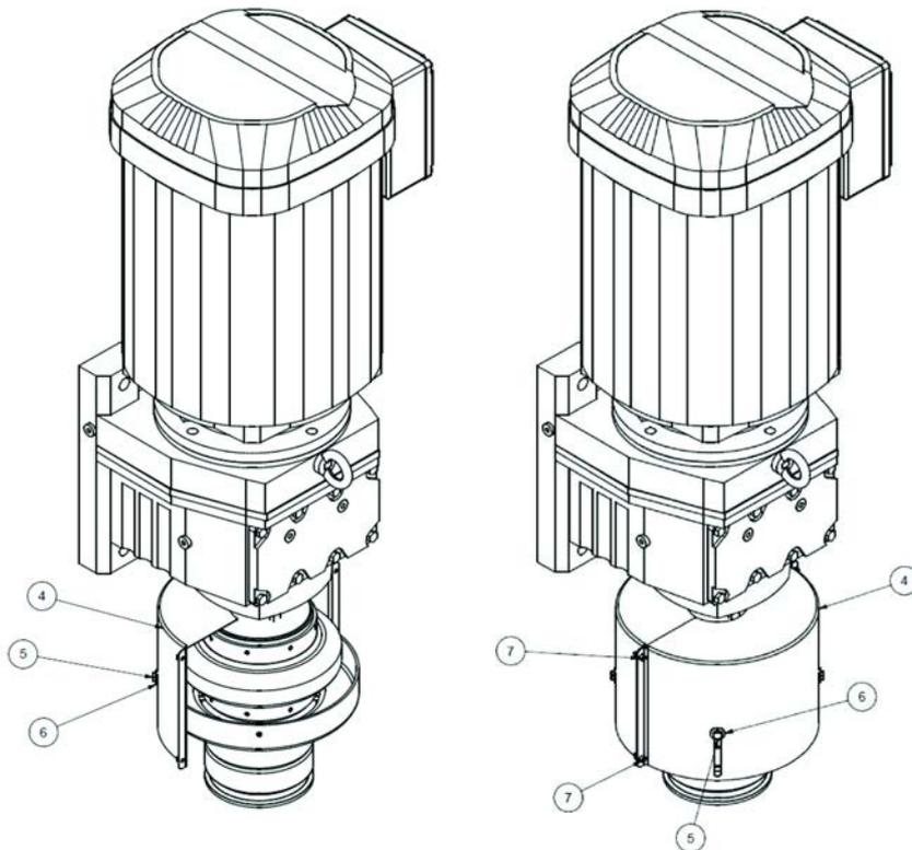
Figure 6-11B Installing the coupling guard continued
