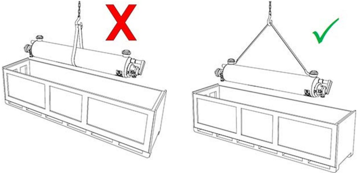
Figure 6-2. Proper Lifting of a Contherm™ from its Crate
