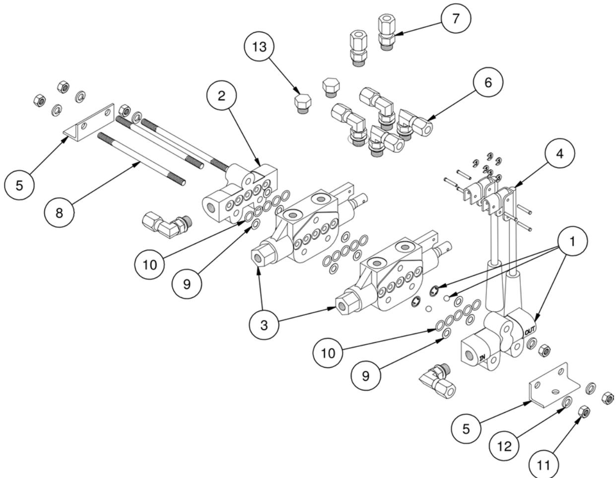
Figure 8-14. Stack Valve Assembly
