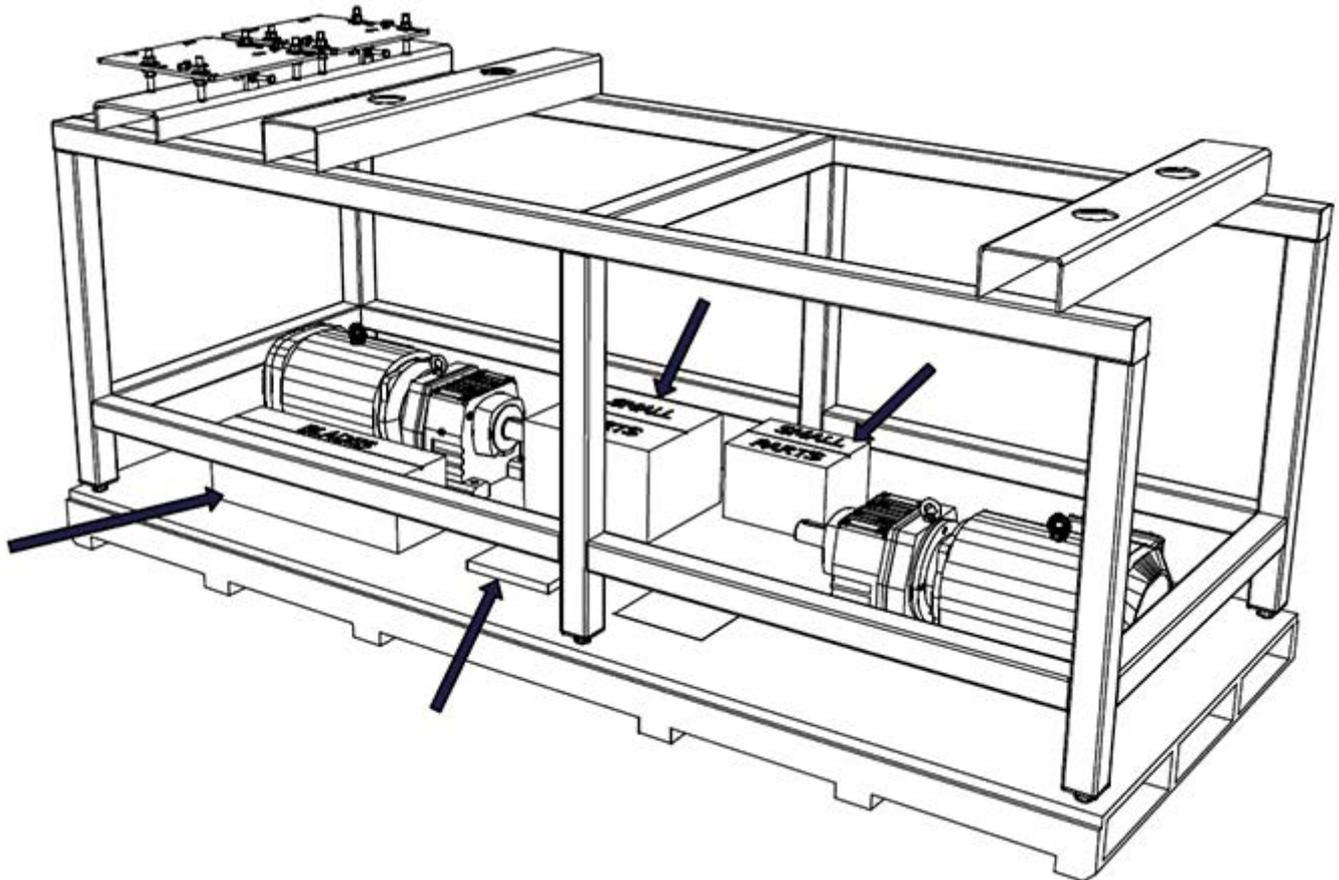
Note: Motor and other important items such as spare parts, blades and documentation will likely be in the crate with the horizontal frame as shown.
