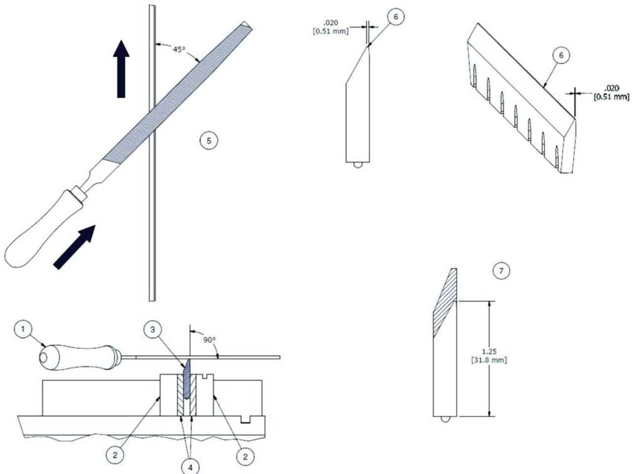
Figure 8-9. Dressing the Contherm™ Scraping Blades
