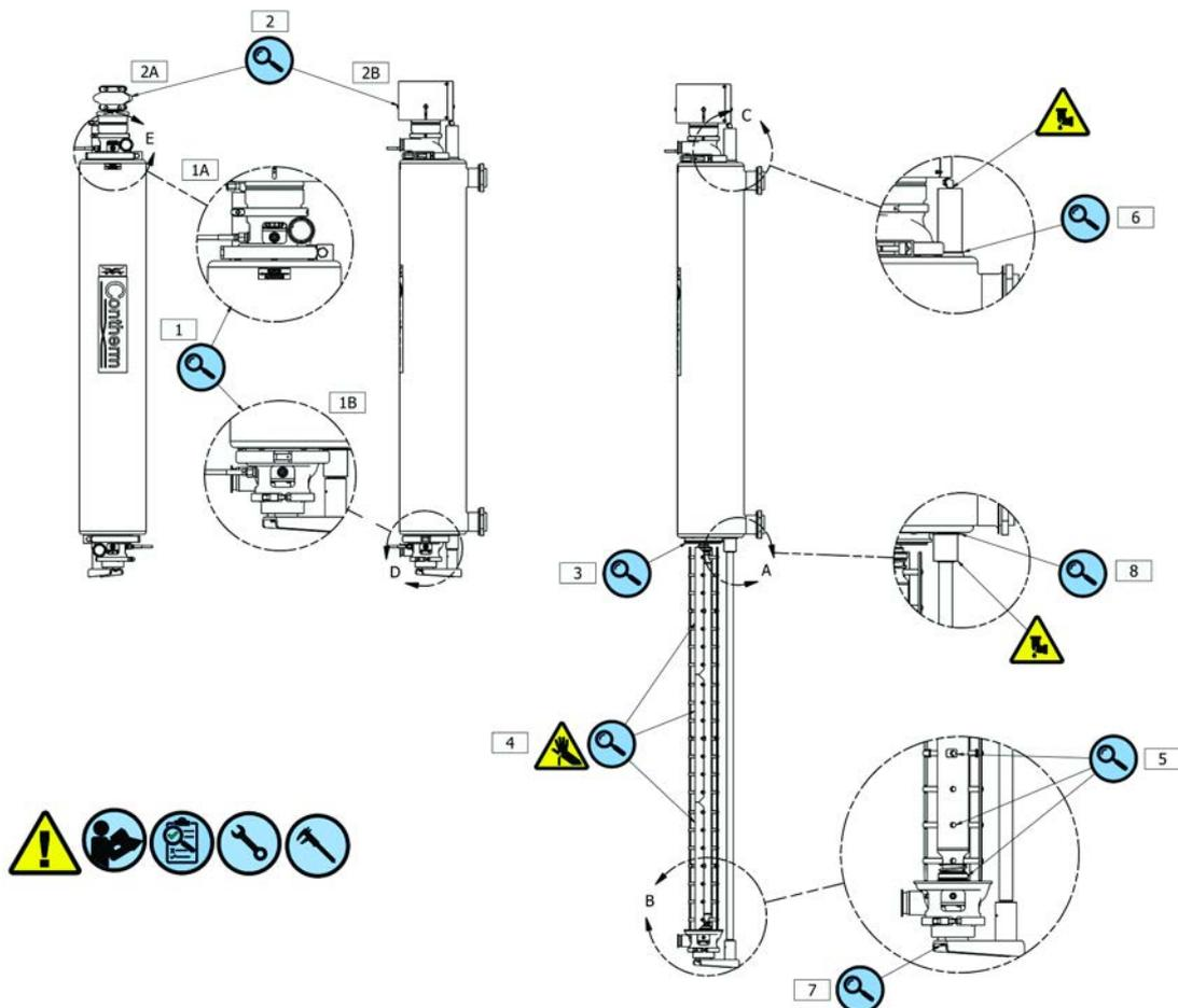
Figure 8-1A Recommended Inspection Points
