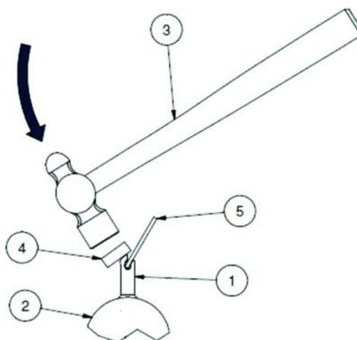
Figure 8-10. Repairing a Damaged Blade Pin
