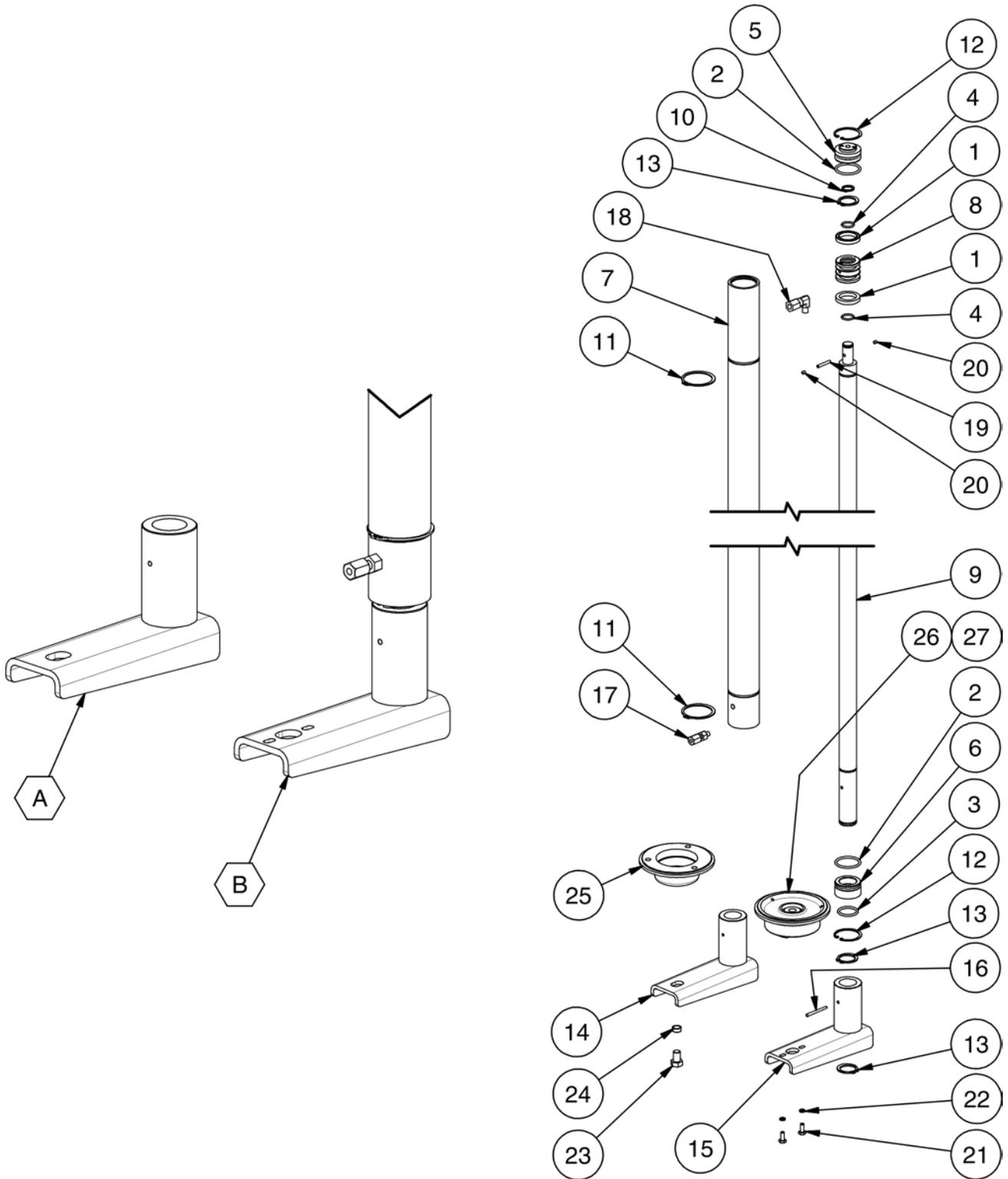
Figure 8-18B . CONTHERM™ Hydraulic Lift Assembly With Hold Down
