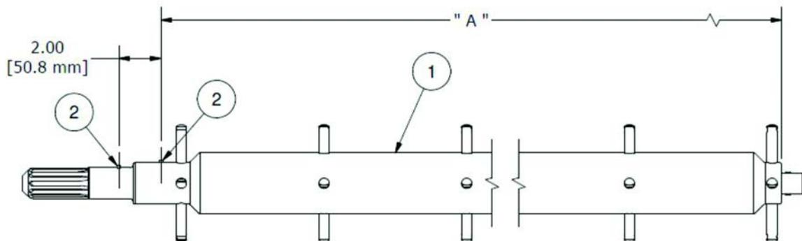
Figure 8-5. Seal Pin Locations for Rotors with Internal Bearings
