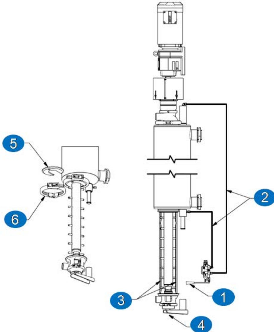
Figure 7-1. Hydraulic Rotor Lift System
