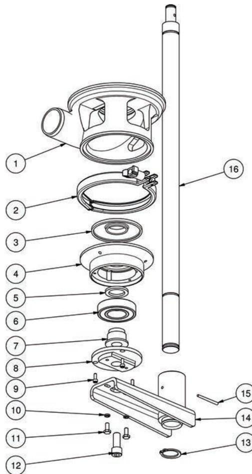
Figure 8-11. Lower Bearings. Non-Hold Down Style
