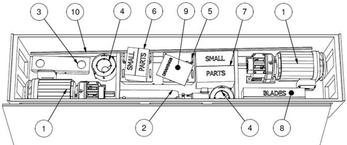
Figure 6-1. Typical Contents of a Crate
