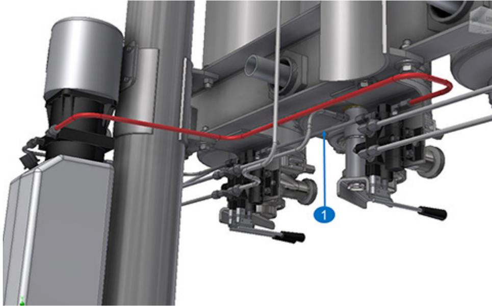
Figure 6-19. Connect Two Stack Valve Assemblies
