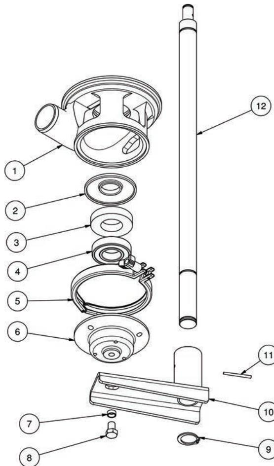
Figure 8-12. Lower bearings, Hold Down Style
