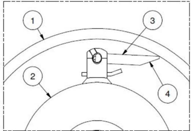
**Figure 8-7. Blade Orientation of Beveled Edge**
