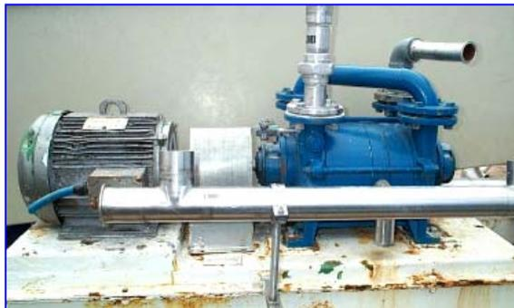
Baldor Motor, 15 hp, 230/460 volt, 38.8/19.4 amsp, 1,760 rpm, 60 Hz. Pump does not have information.
