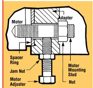
**Unique C-Plus Precision Alignment System (Four Point)**
