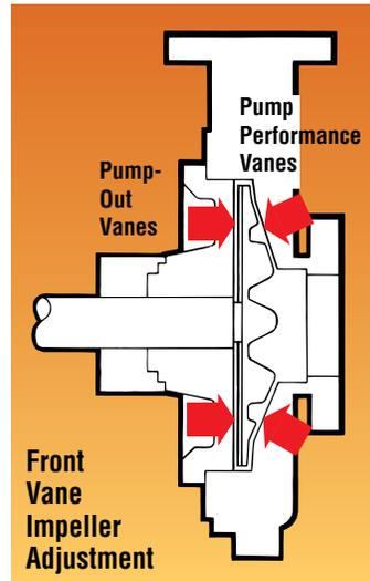
**Performance Life Cycle: Front Vane Open Style Impeller with Pump Out Vanes**
