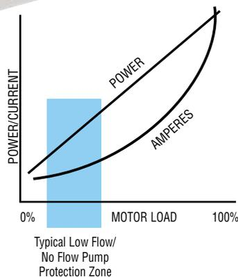
**By Sensing Power** and not just amperes, linear measurements are provided with the sensitivity to detect improper operation while eliminating unwanted nuisance trips
