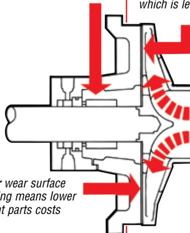
*Lowest Overall required NPSH of any standard pump*
