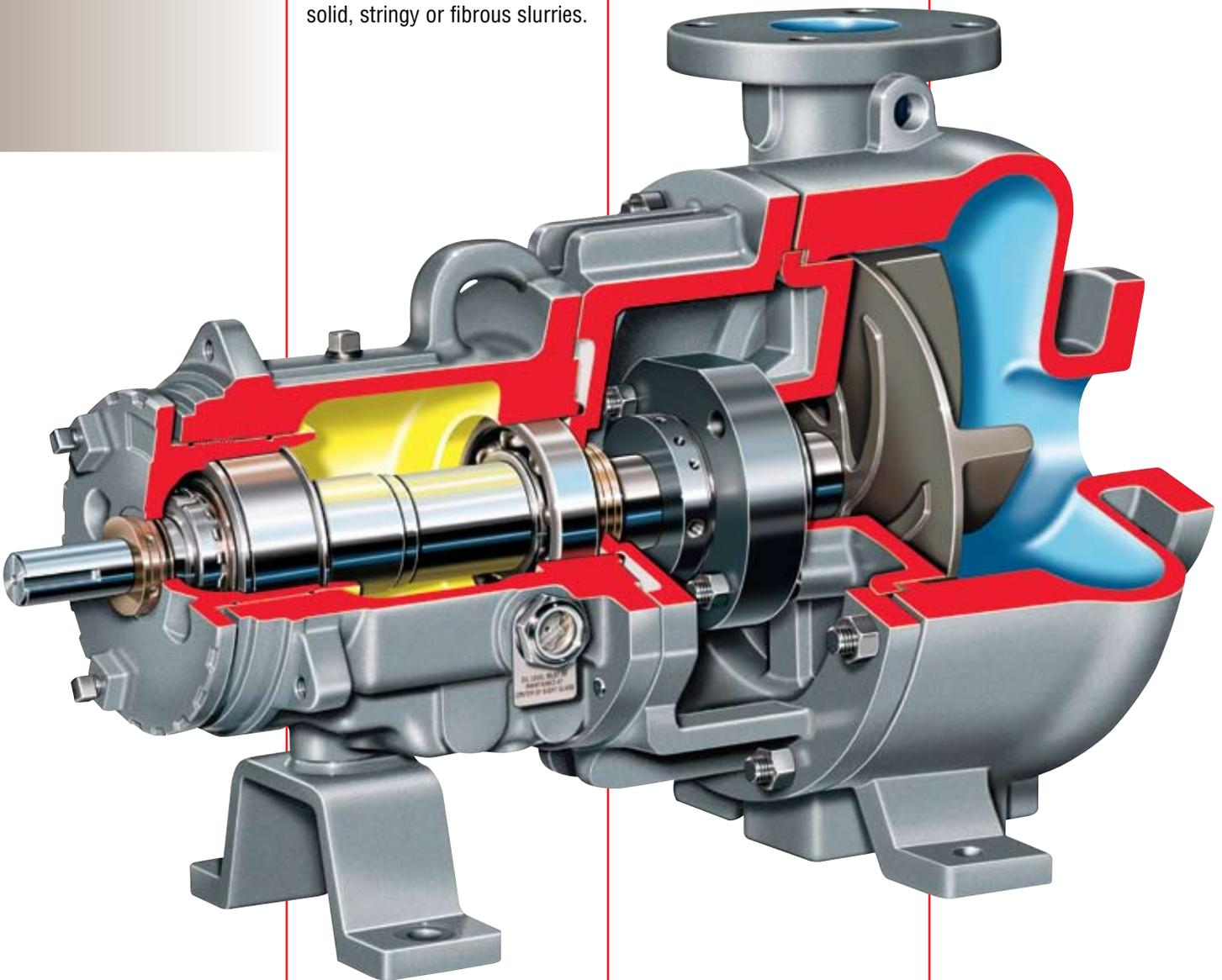
**Vortex Action** minimizes abrasive wear while maintaining solids integrity because only a fraction of the media contacts the impeller
