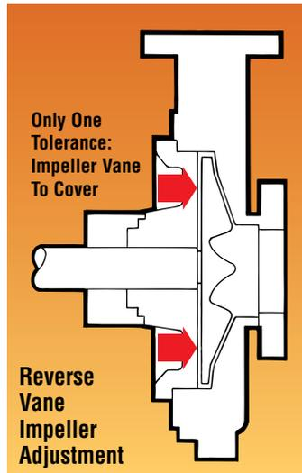
**Performance Life Cycle: Durco Reverse Vane Impeller with Balance Holes**
