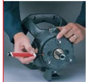
Select the impeller setting. Each notch on the carrier ring represents exactly 0.10 mm (0.004 in) of clearance. For an impeller setting of 0.5 mm (0.020 in) count five notches counterclockwise.
