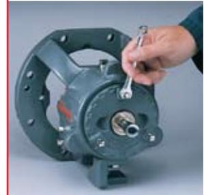
Simply loosen the setscrews. Using a wrench rotate the bearing carrier counterclockwise until the impeller lightly touches the rear cover plate.
