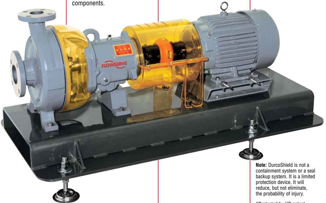
**Note:** DurcoShield is not a containment system or a seal backup system. It is a limited protection device. It will reduce, but not eliminate, the probability of injury.
