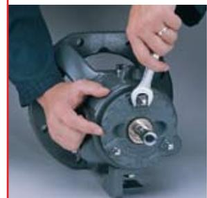
Move the bearing carrier clockwise the selected number of notches. Tighten the setscrews and check the impeller clearance with the feeler gauge.
