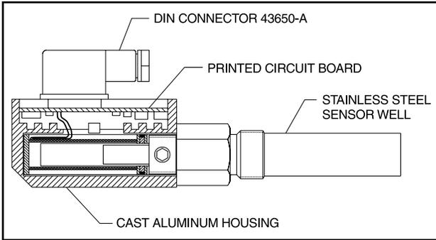
Figure 41. Volume Ratio Control Transmitter
