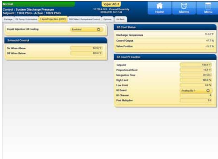
**Figure 20. Liquid Injection Adjustment Screen**
