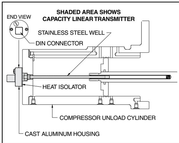
**Figure 40. Capacity Linear Transmitter**
