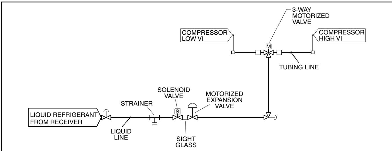
**P & I DIAGRAM, LIQUID INJECTION - DUAL PORT (OLD DESIGN)**
