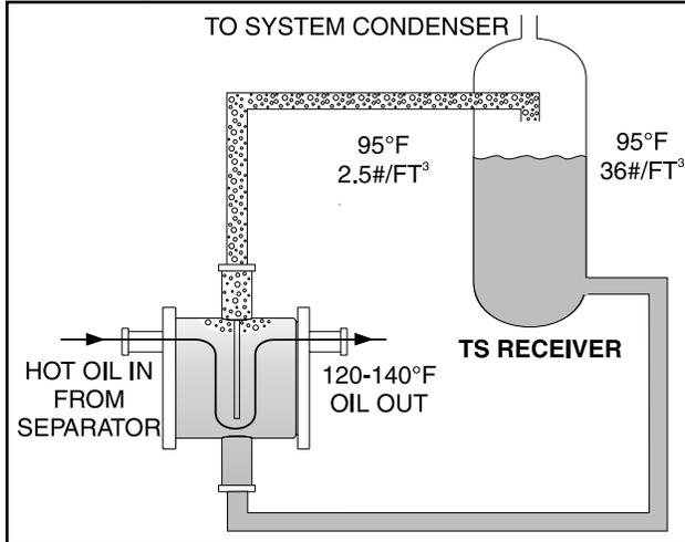
**Figure 4. Thermosyphon Receiver System**
