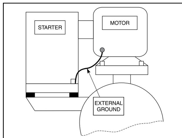
Figure 46. Motor And Starter Grounding
