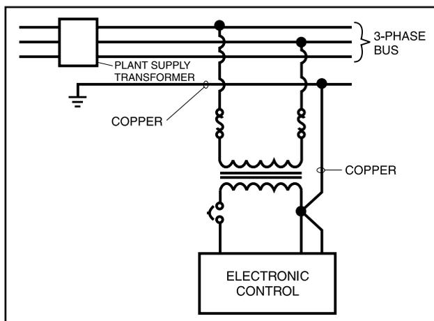
Figure 45. Control Power Ground Circuit
