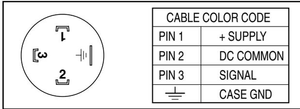
**Figure 39. Pressure Transducer Color Key**
