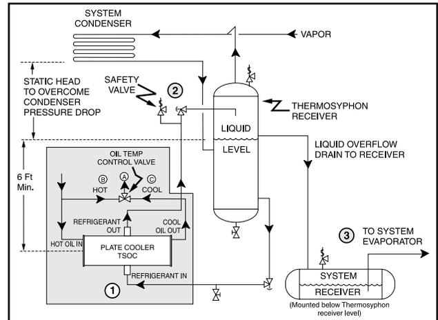
**Figure 5. TSOC Piping Arrangement**
