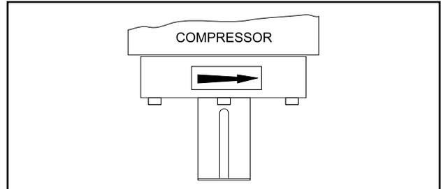
**Figure 15. Shaft Rotation Direction**
