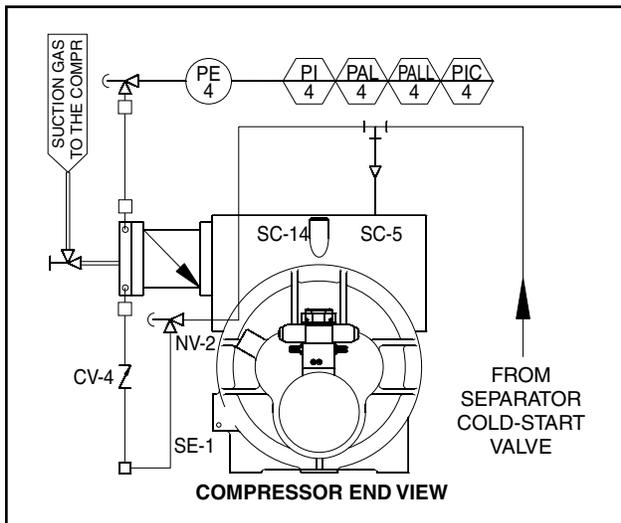
Figure 26. Suction Check Valve Bypass
