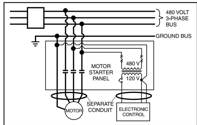
**Figure 47. Separation Of Different Voltage Circuits**
