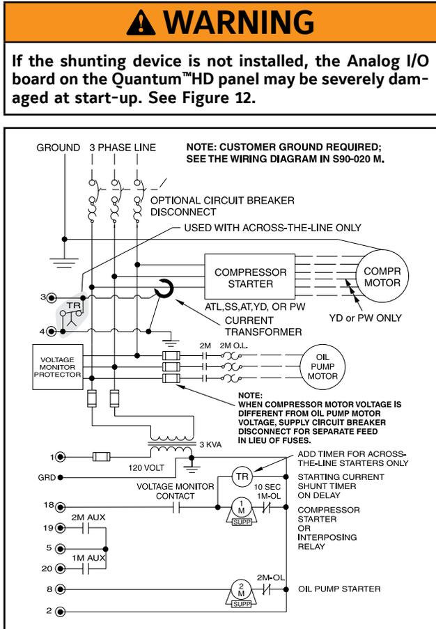
Figure 12. Starter Wiring Diagram
