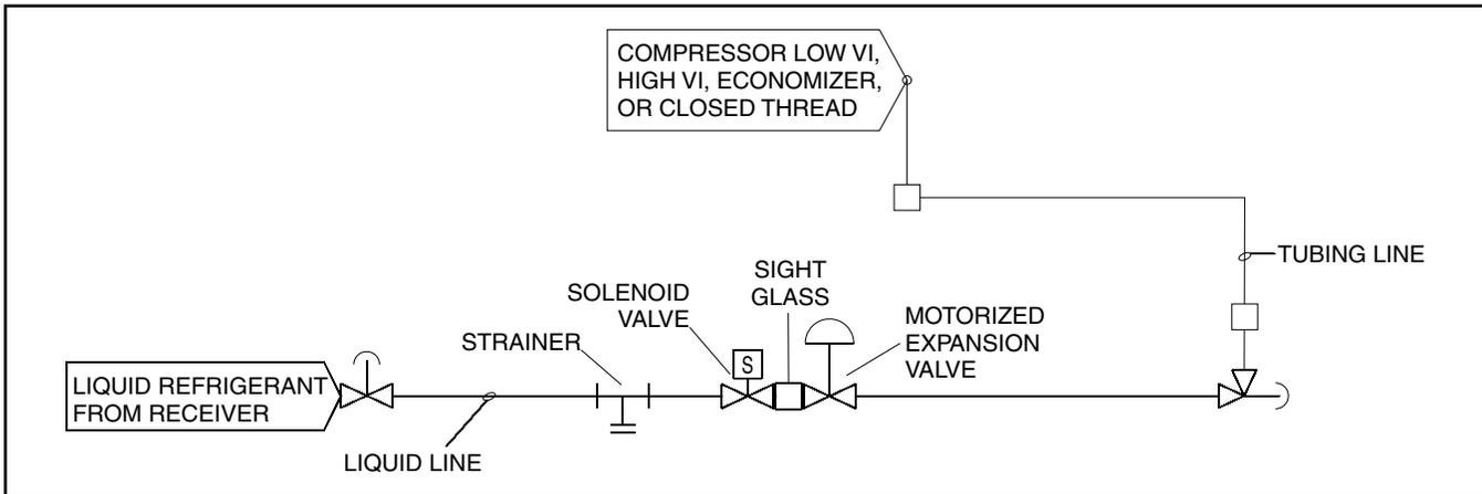
**P & I DIAGRAM, LIQUID INJECTION - DUAL PORT (NEW DESIGN)**
