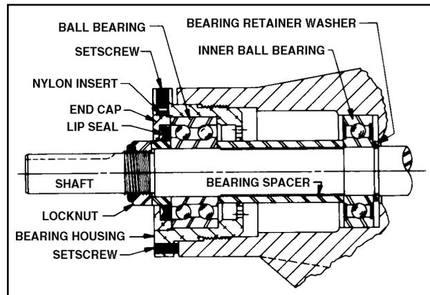
Figure 32. Thrust-Bearing assembly (AS, AK, AL)
