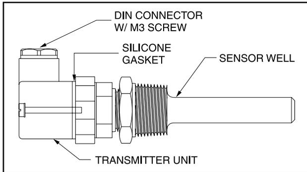
Figure 42. Temperature Transmitter
