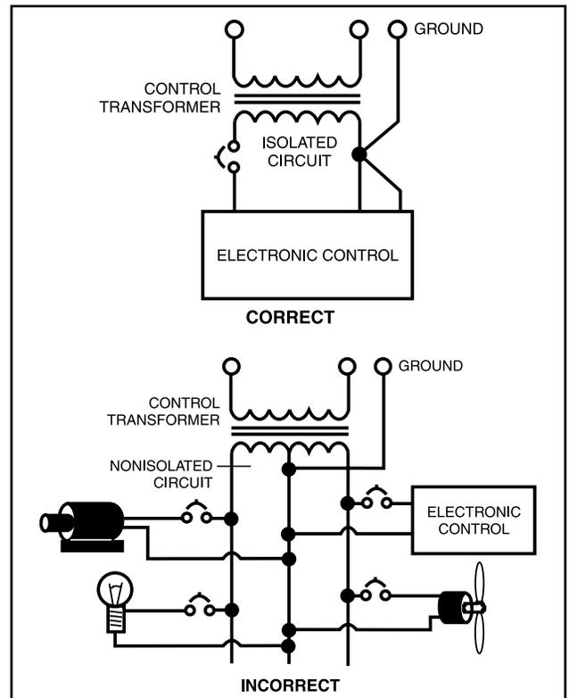
Figure 44. Voltage Source Circuit To Prevent EMI
