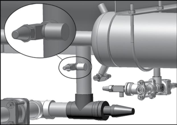
Figure 2. Oil Drain Valve
