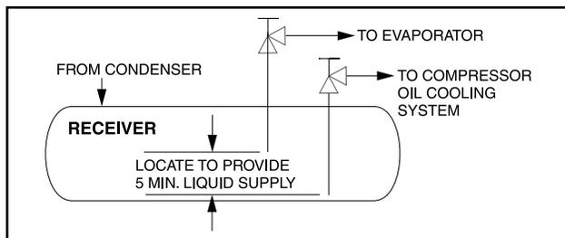
Figure 6. Dual Dip Tube
