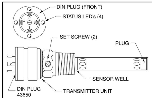
Figure 43. Oil Level Transmitter
