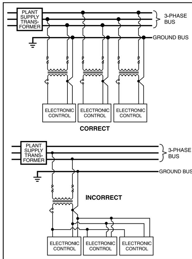
Figure 48. Electronic Control Panel Power Supplies
