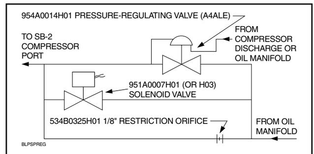
Figure 28. High-Stage SB-2 Oil Supply Line Diagram
