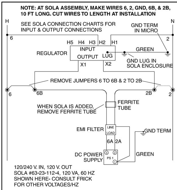
Figure 14. Recommended Regulator Installation
