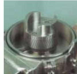
The rotor grinding element is mounted directly on the motor shaft. The grinding gap can be adjusted steplessly. The gap width can be read off on a scale and reproduced at any time.
