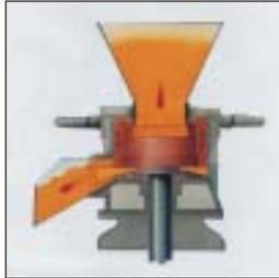
The product is fed to the mill either openly via a hopper or by means of a pump in a closed pipeline system. A special toothed-colloid grinding set with an adjustable grinding gap is used for the grinding or homogenization process. Different grinding sets can be used, depending on the product.
