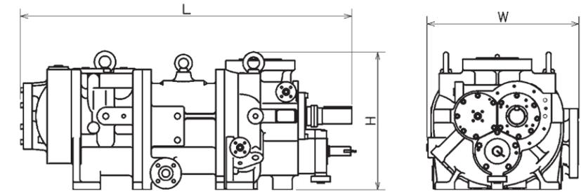
\* The outer dimension drawings illustrate the model GH250L.
