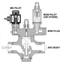
forces the main valve seat to open wide to permit flow in the direction of arrow.
