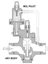
and outlet pressure. Increased range spring force increases the differential setting. Inlet pressure, counteracted by the range spring plus outlet pressure, enters the space on top of the piston which forces the main valve seat to open and regulate flow. The external sensing tube on the 5" & 6" valves must be customer supplied and field installed.
