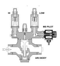
the HA4A regulator. When inlet pressure rises above the higher setting, the control module opens to allow inlet pressure to enter the space on top of the piston which forces the main valve seat to open and regulate flow. Typically used as a combined evaporator pressure regulator and defrost internal relief valve.
