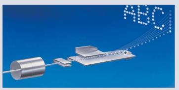
Ink jet printing is carried out by electronically controlled ink drops to ensure perfect printing positioning.
