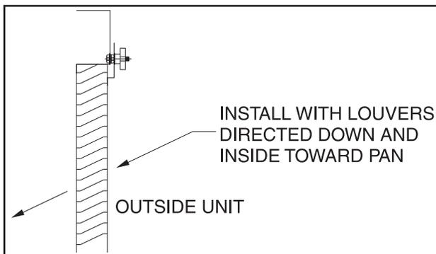
Figure 2-3. Louver Installation
