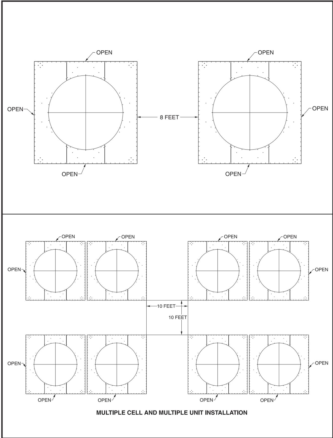
Figure 1-2. IDC Unit-to-Unit Spacing Requirements
