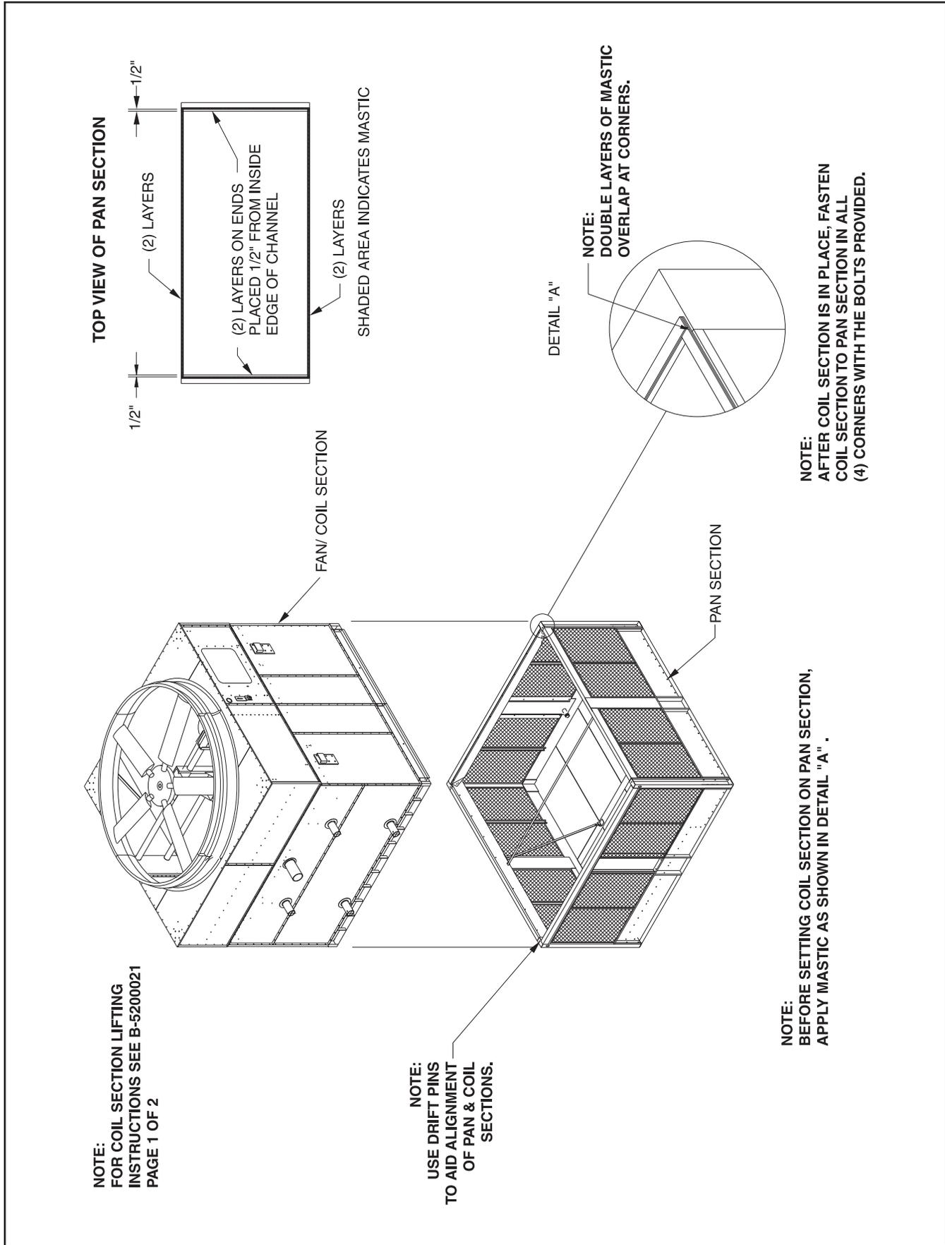
Figure 2-4b. Assembly and Placement
