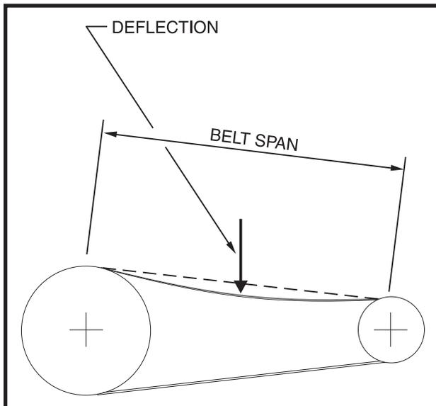
Figure 4-5. Belt Tensioning Schematic
