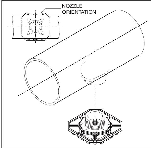
**Figure 4-6. Spray Header Nozzle Orientation**
