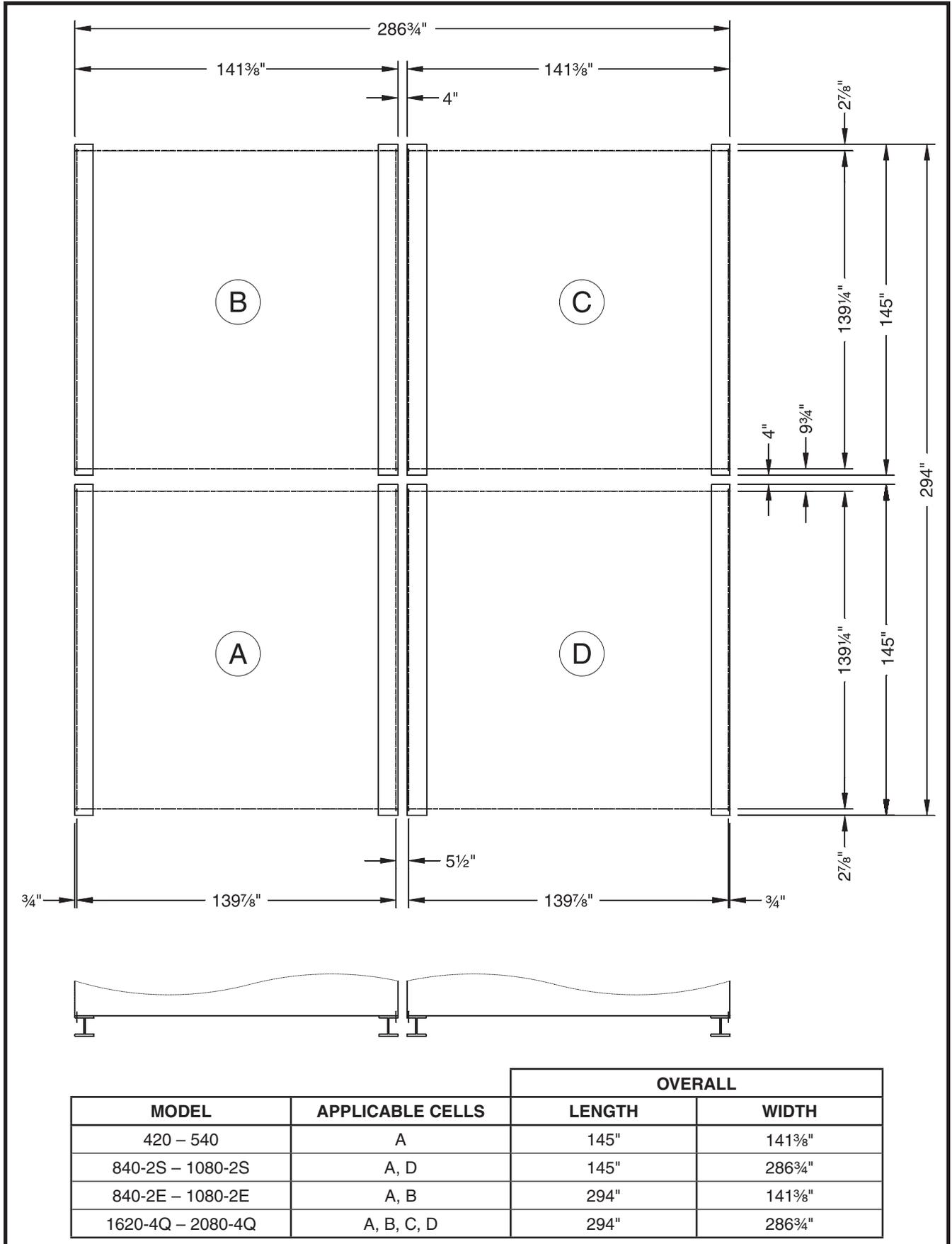
Figure 2-1a. 12' x 12' Foundation Layout
