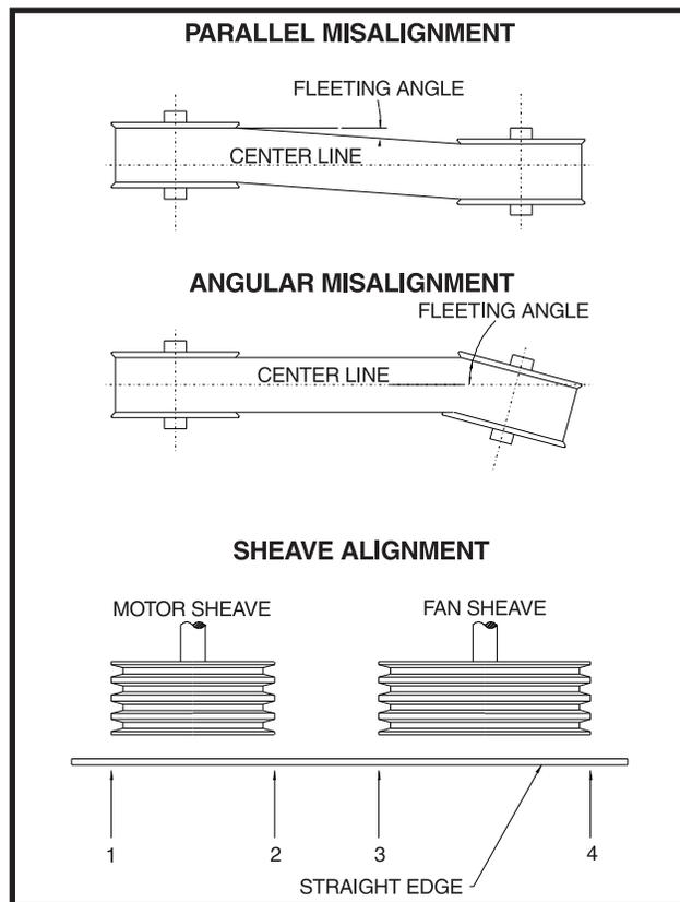
Figure 4-3. Sheave Alignment
