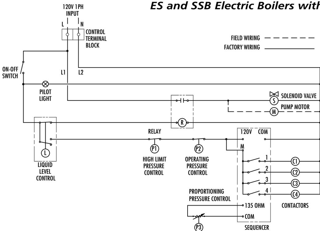
**ES Electric Boiler with Auxiliary Low Water Cutoff**
