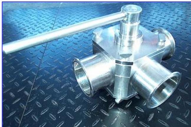
*Working Principle: A polytetrafluoroethylene (PTFE) shutter is operated by means of a handle or an actuator. A spring washer system presses the shutter against the internal cylindrical surface of the valve body, ensuring a tight seal.*
