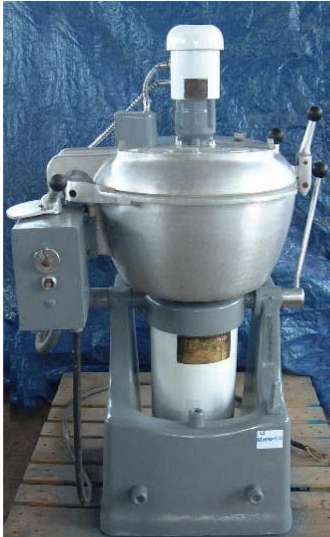
For high speed cutting, mixing, and blending.
