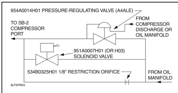
Figure 7. Pressure Regulating Valve
