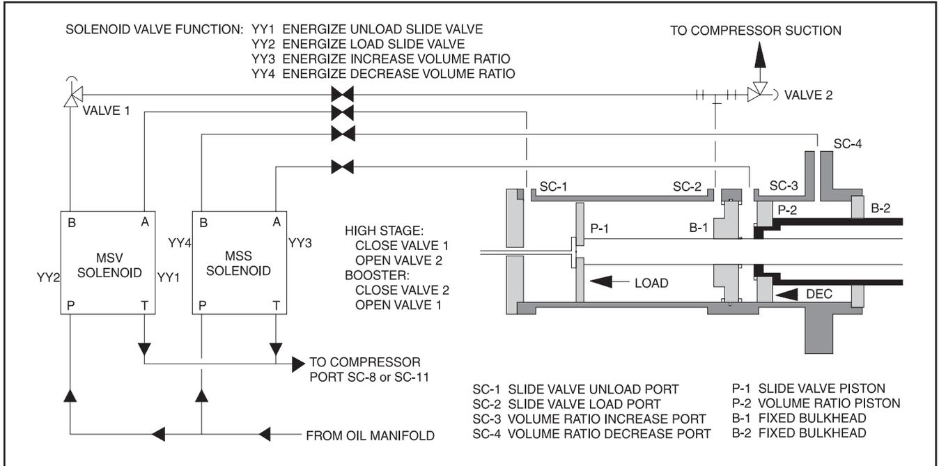
MSV and MSS HYDRAULIC CYLINDER and SOLENOID VALVES
