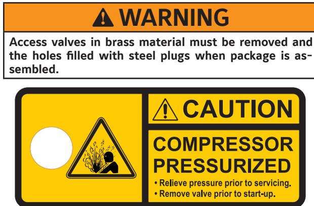
**Figure 4. Caution/Identification Tag on Access Valve**
